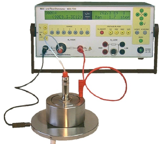
Measurement of surface resistance with base plate GP 14 and Milli-TO 3
